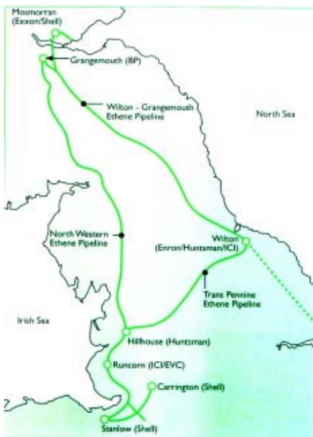
Figure 1.4 Ethene pipelines connect refineries and chemicals plants in the UK . Annual production of ethene is 2.1 million tonnes in the UK and over 80 million tonnes in the rest of the World. (from The Essential Chemical Industry )
